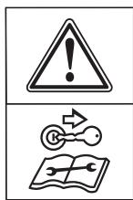
Before beginning any work on this mower, remove the ignition key and observe all information contained in these instructions.
