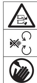
Injury hazard due to rotating blades or other moving parts. Keep hands and feet out of the openings when the machine is running.
